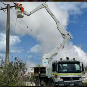
Make Sherrin Equipment 18GB Model Tare Weight (KG) 10200 Width (MM) 2490 8685 Length (MM) 4200 Height (MM) Reach (Metres) 11.1 Safe Work Load 350 Working Height (Metres) 18 Chassis 4x2, 4x4, 6x4 132kV **Insulation** Rating
